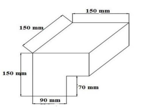
Figure.3: Shear plane 150\*80 mm
