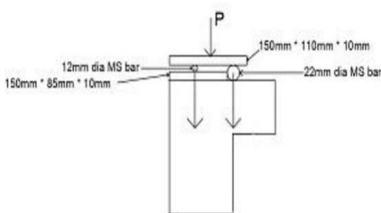
Figure.1: Shear strength test setup
