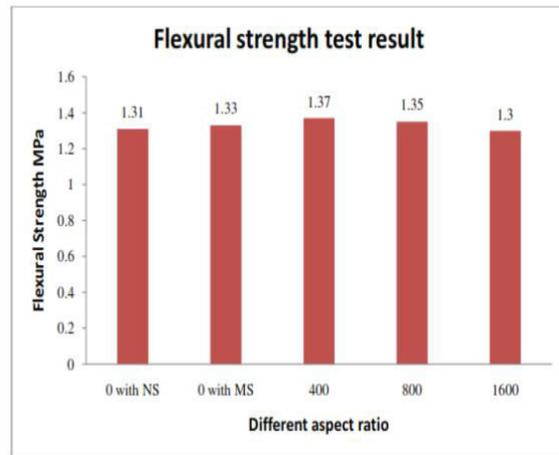
Figure.6: The variation of 28days theoretical Flexural strength test results
