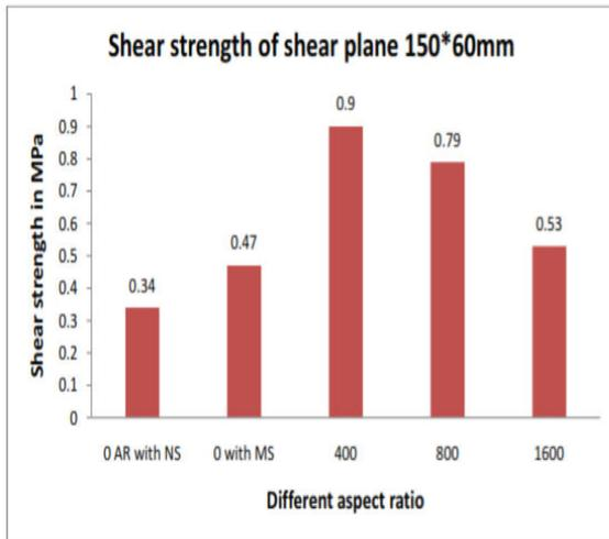
Figure.9: The variation of shear strength test results (shear plane 150\*60)
