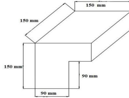
Figure.4: Shear plane 150\*60 mm
